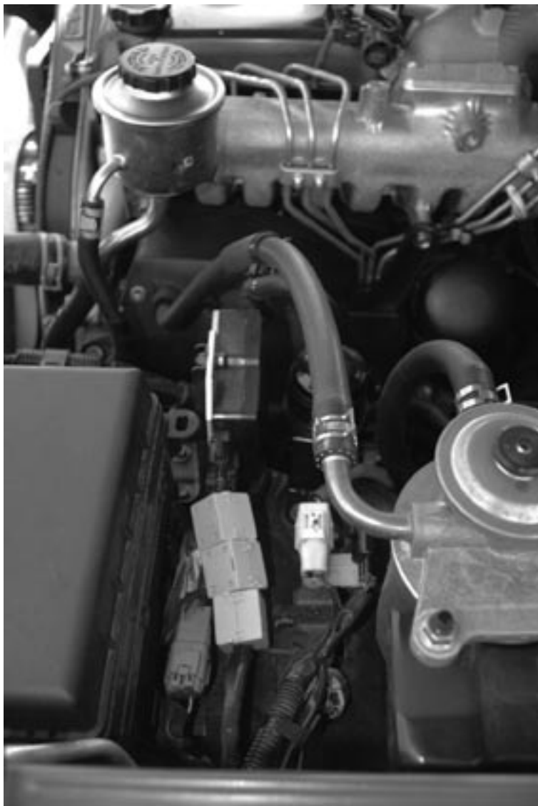
You can see the white beads placed on the cable coming from the injectors.
